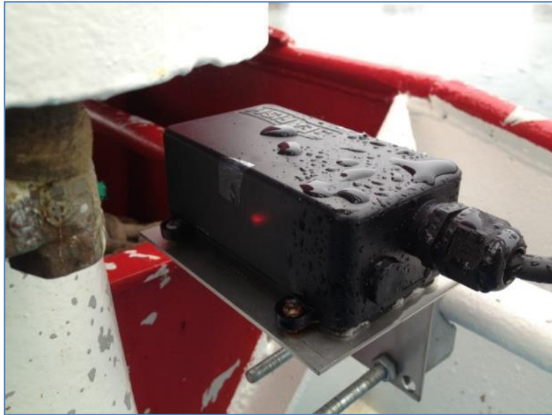
Figure 5. SC2 iVMS system fitted to a small fishing vessel
